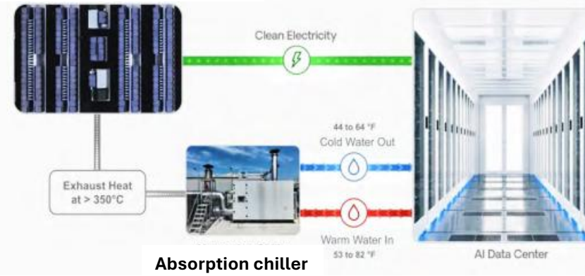
200 MW onsite Heat Capture-Enabled fuel cells
